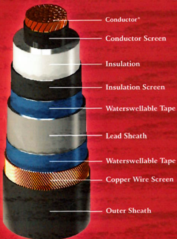
LEAD SHEATHED COPPER WIRE SCREENED CABLE
