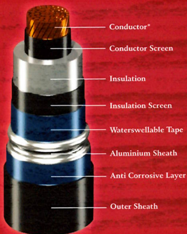
CORRUGATED ALUMINIUM SHEATHED CABLE
