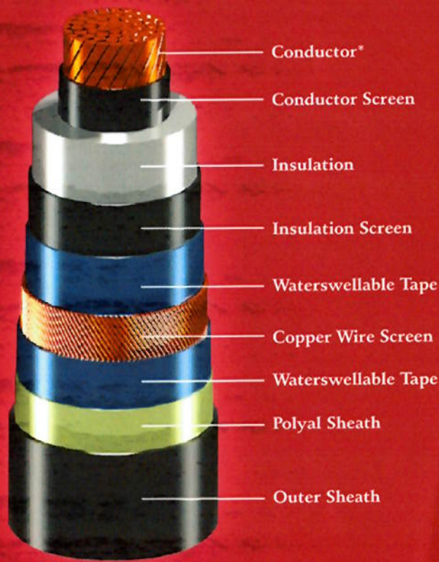
COPPER WIRE SCREENED POLY-AL TAPE CABLE
